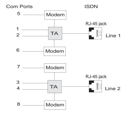
From the perspective of the server PC, the ISIHI-2S is an 8-port serial card with eight devices permanently attached to the serial ports. The first four ports are the two terminal adapters, each of which appear as two ports. The remaining four ports are the four central site modems. The chart below summarizes the correlation of ports and devices.
